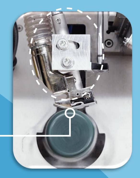
Socks cleaning and reversing machine; this machine has been produced for cleaning the long yarn pieces on the socks and reversing them finally.
